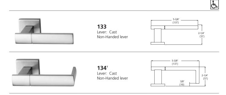
Complies with codes requiring lever to return to within 1/2" (13mm) of door face.
